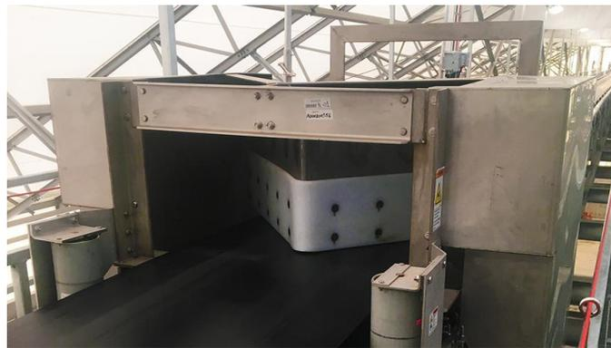
GSI InterSystems fertilizer plow conveyor provides a highly efficient alternative to traditional conveyor systems, according to the company.
